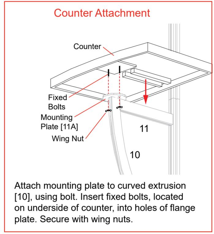
Keep mounting plate [11A] and wing nuts attached to counter, when packing.
