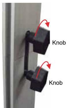
Slide connection bar between extrusions, then turn knobs clockwise to tighten lock.
